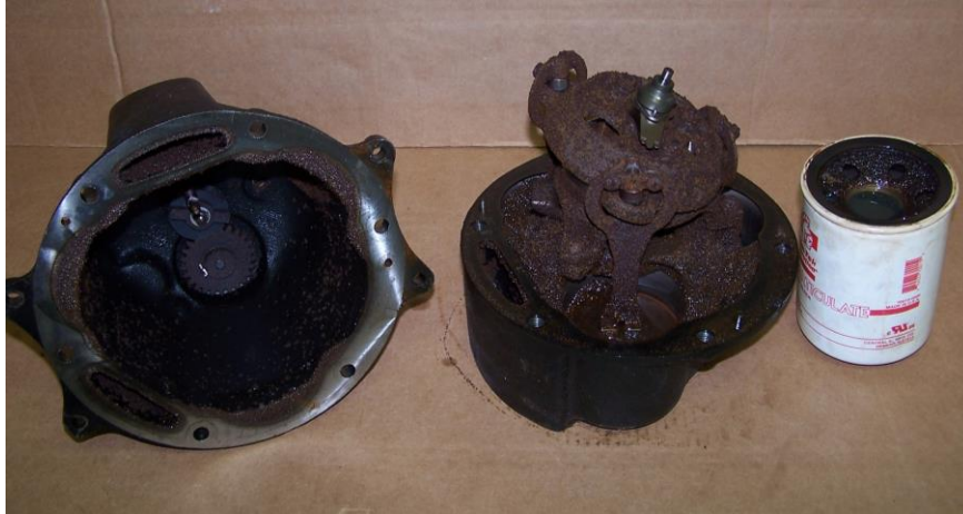
Diesel Fuel Storage Tank Pump/Meter Assembly and Island Filter With Corrosion From Fuel
