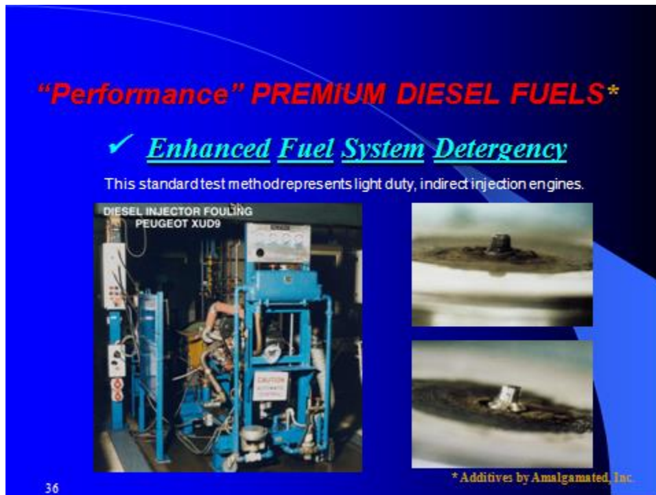
Peugeot XUD9 Fuel Injector Test Apparatus & Test Injector Tip Photos
