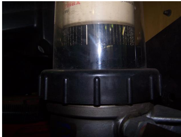
Diesel Engine Fuel Filter With Black (Unstable) Fuel Creating Asphaltenes After Only 30 Minutes Of Operation
