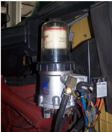
Diesel Engine Fuel Filter With Black (Unstable) Fuel Creating Asphaltenes After Only 30 Minutes Of Operation
