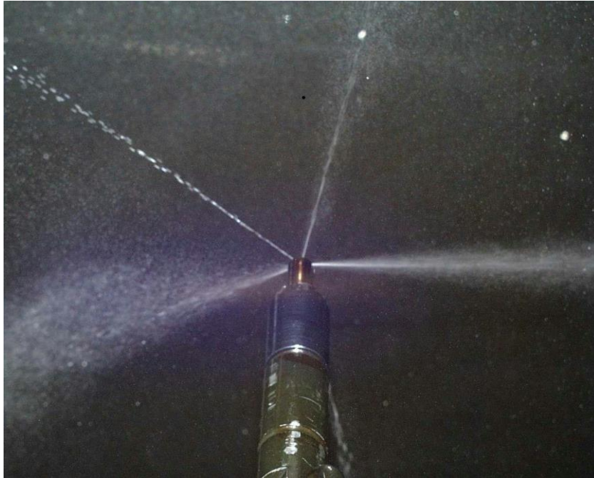
Diesel Injector Spray Pattern With Partially Plugged Tip Holes (Uneven Spray Pattern)
